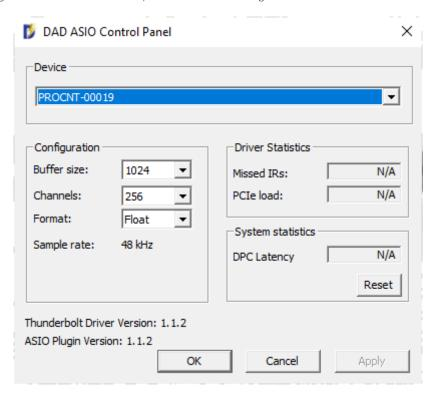
Figure 5: ASIO driver configuration window
