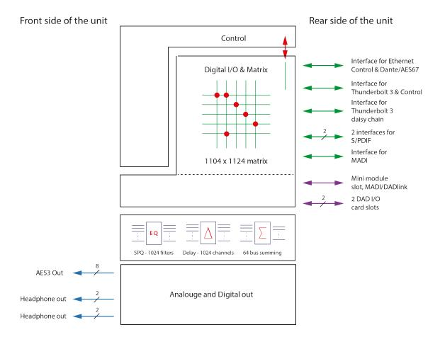
Figure 1: Block diagram of the unit
